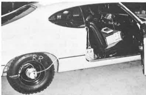
Figure 20. Test equipment used for dynamic-force measurements.
