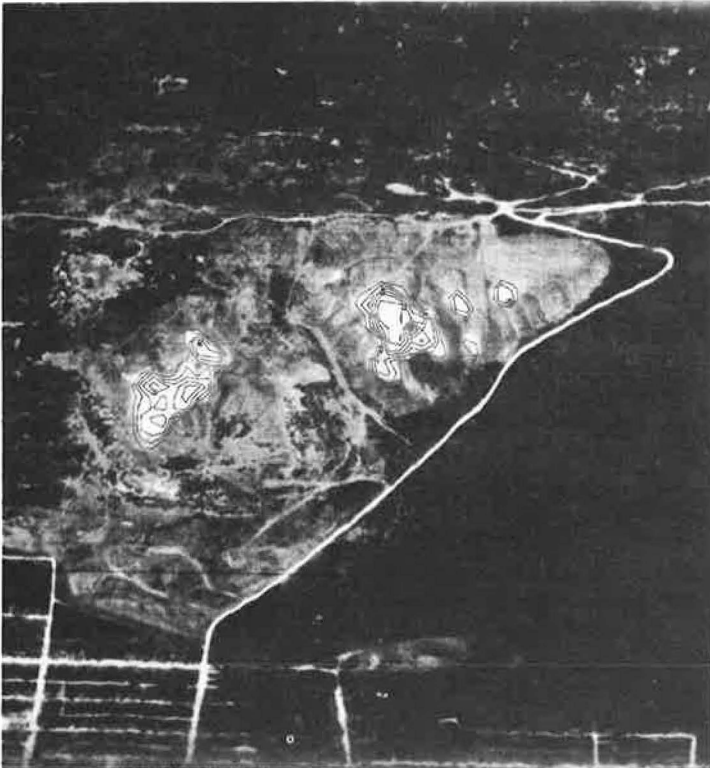
Figure 6. Computer-generated thermal contour lines overlaid on a thermal image of a burning coal refuse bank in Pennsylvania.
