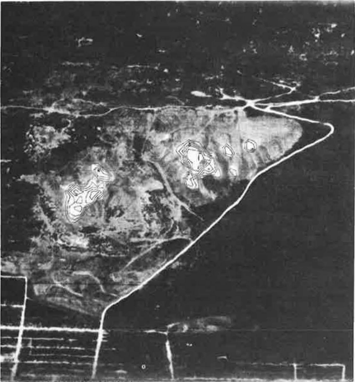
Figure 6. Computer-generated thermal contour lines overlaid on a thermal image of a burning coal refuse bank in Pennsylvania.
