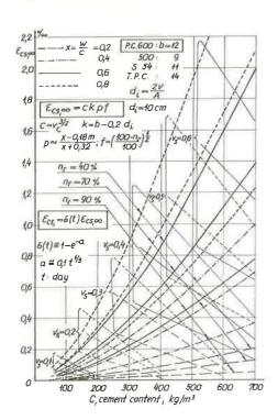
Figure 7. Effects on shrinkage of a concrete of cube strength  $f_c = 245 \text{ kip/cm}^2$  (3,500 psi).
