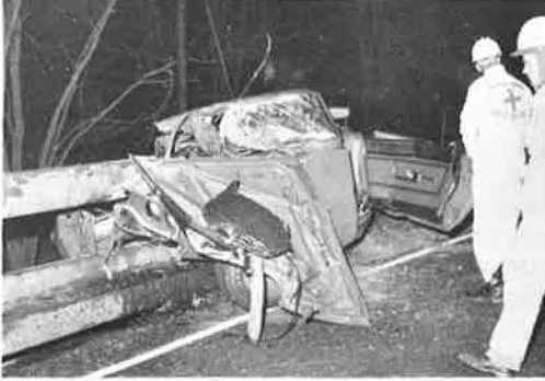
Figure 7. Head-on collision with right end post of bridge shown in Figure 6.
