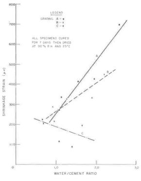
Because of the importance of the strain at break in the structural design of lean-mix concrete bases, part of the second phase of the laboratory study was aimed at investigating the effect of grading on this and other engineering properties of lean-mix concrete.
