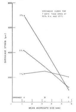
Figure 14. Relation between shrinkage strain and w-c ratio of lean-mix concrete gradings A, B, and C.
