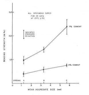
Figure 5. Relation between bending strength and mean aggregate size for lean-mix concrete.
