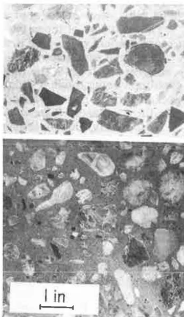
Figure 4. Crushed stone and gravel concretes.
