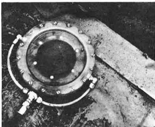
Figure 5. Pressure cell before installation.
