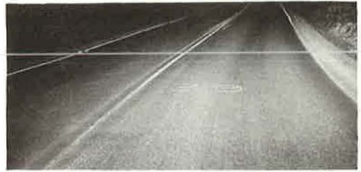
Figure 7. 0.010-in. beaded test line (left) and standard reference line (right).
