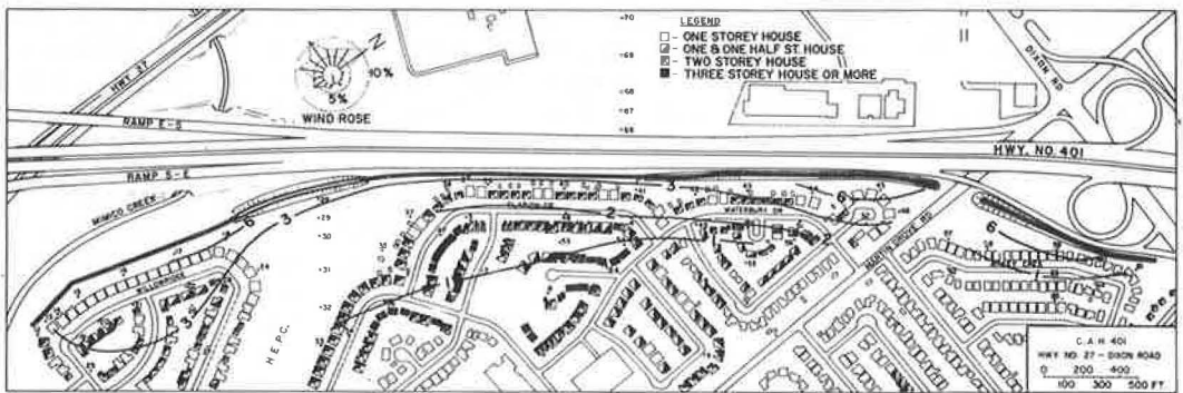
Figure 11. Measured reductions of sound levels ( L_{10} ) due to Highway 401 barrier.
