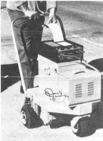
Figure 3. Instrument developed to detect delamination on bridge decks.
