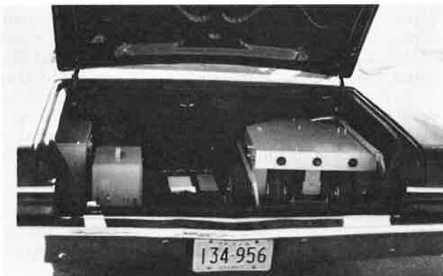
Figure 10. Delamination detector disassembled and stowed in an automobile trunk.
