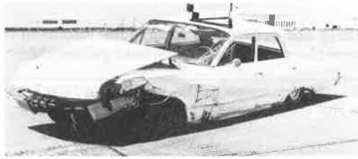
Figure 20. Vehicle damage after CMB-4 test.
