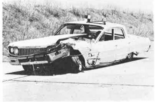
Figure 16. Vehicle damage after CMB-2 test.
