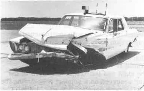
Figure 6. Vehicle damage after MBGF test.
