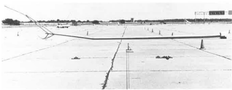
Figure 14. Light pole after test LS-3.
