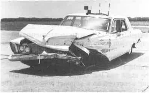
Figure 6. Vehicle damage after MBGF test.
