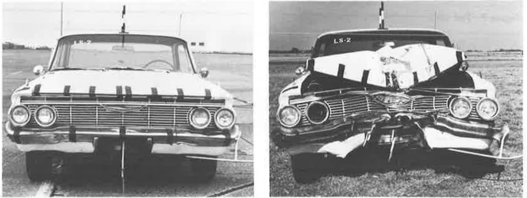
Figure 9. Front of vehicle before and after test LS-2.
