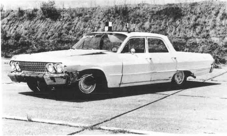
Figure 18. Vehicle damage after CMB-3 test.
