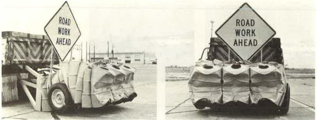
Figure 8. Crash-cushion trailer after test.
