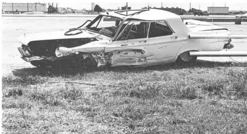
Figure 10. Vehicle damage after E-3 test.
