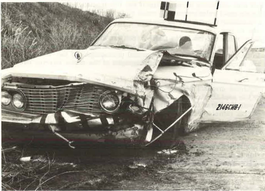
Figure 13. Vehicle damage after CMB-1 test.
