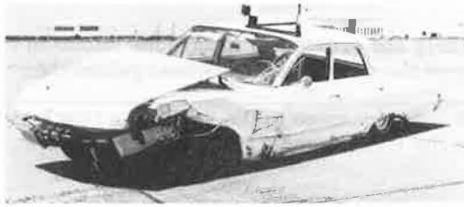
Figure 20. Vehicle damage after CMB-4 test.
