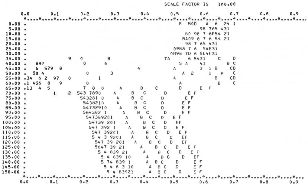
Figure 10. Speeds in severe incident: \alpha = 20 and \gamma = 0.51 (service = 7.399E + 0.3 vehicle-miles; 50-mph delay = 1.049E + 0.3 vehicle-miles).
