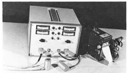
Figure 3. Pavement displacement measuring system.
