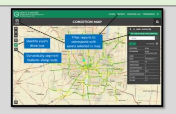
Condition maps provide network level screening based on color coded features, and to allow access to detailed asset information through an "Asset Inspector" tool.
