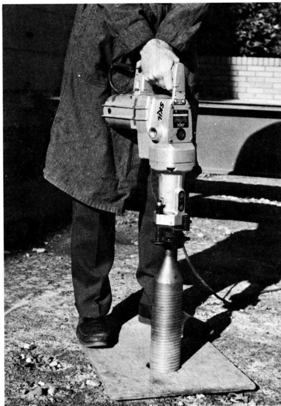
Figure 11. Coring device used in conjunction with Rainhart volumeter for density tests on soils and granular bases.
