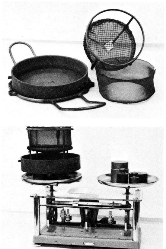
Figure 4. Weighing pan and sample basket. Disassembled basket and pan with carrying frame (upper). In weighing position (lower).
