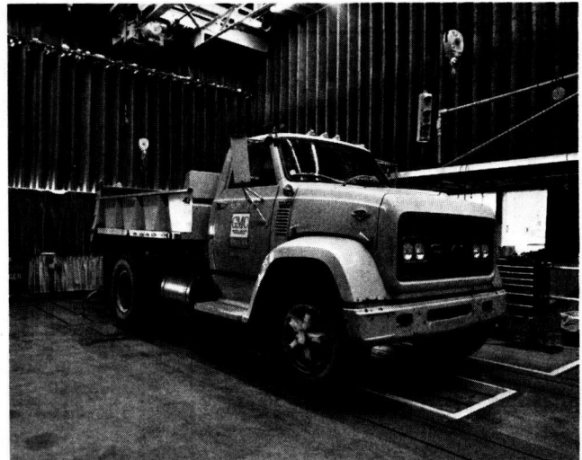
Figure M-3. Test Vehicle No. 1 on chassis dynamometer.
