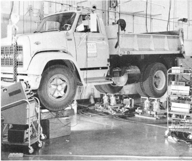
Figure 10. Test Vehicle No. 1 on hydraulic servo rams.
