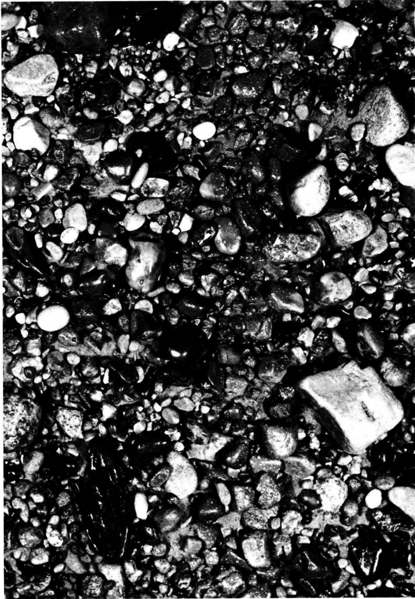
Figure 53. The bed when a riprap having the same effective size as the previous photos (0.073 ft), but with a standard deviation, \sigma , of 2.7, is placed on the bed prior to the test. The extreme range of sizes found in this mixture is characteristic of material with a high standard deviation. In this test the riprap layer was only one diameter thick; again, base material can be seen between the interstices at various points on the bed.
