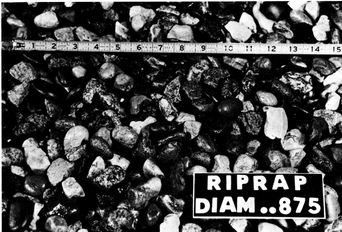
Figure 48. Uniform riprap material as placed on the channel bed and subjected to the design flow. The effective diameter, d_{50} , equals 0.073 ft (0.875 in.). The standard deviation of this material based on the sieve limits is 1.07. The thickness of this riprap layer is equivalent to three times the effective diameter.
