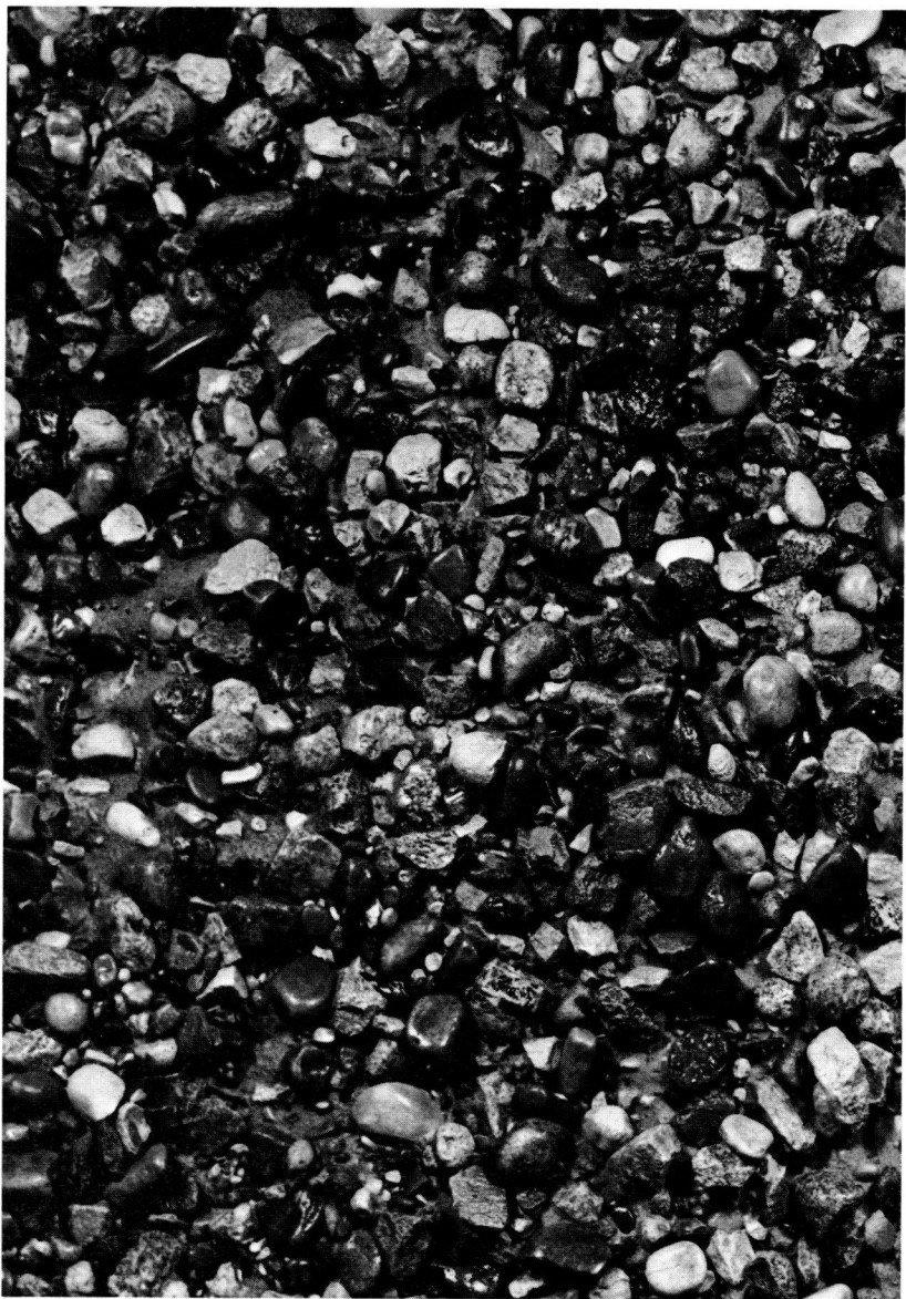
Figure 49. Riprap material having an effective size, d_{50} , equal to 0.073 ft but a standard deviation of 1.5. The standard deviation is a measure of the spread of the particle gradation, and the larger the standard deviation, the wider is the range of particle sizes. This is apparent by comparing Figure 49 with Figure 48. Here the layer of riprap material is only one diameter thick, so base material is exposed at various points through the interstices of the riprap.
