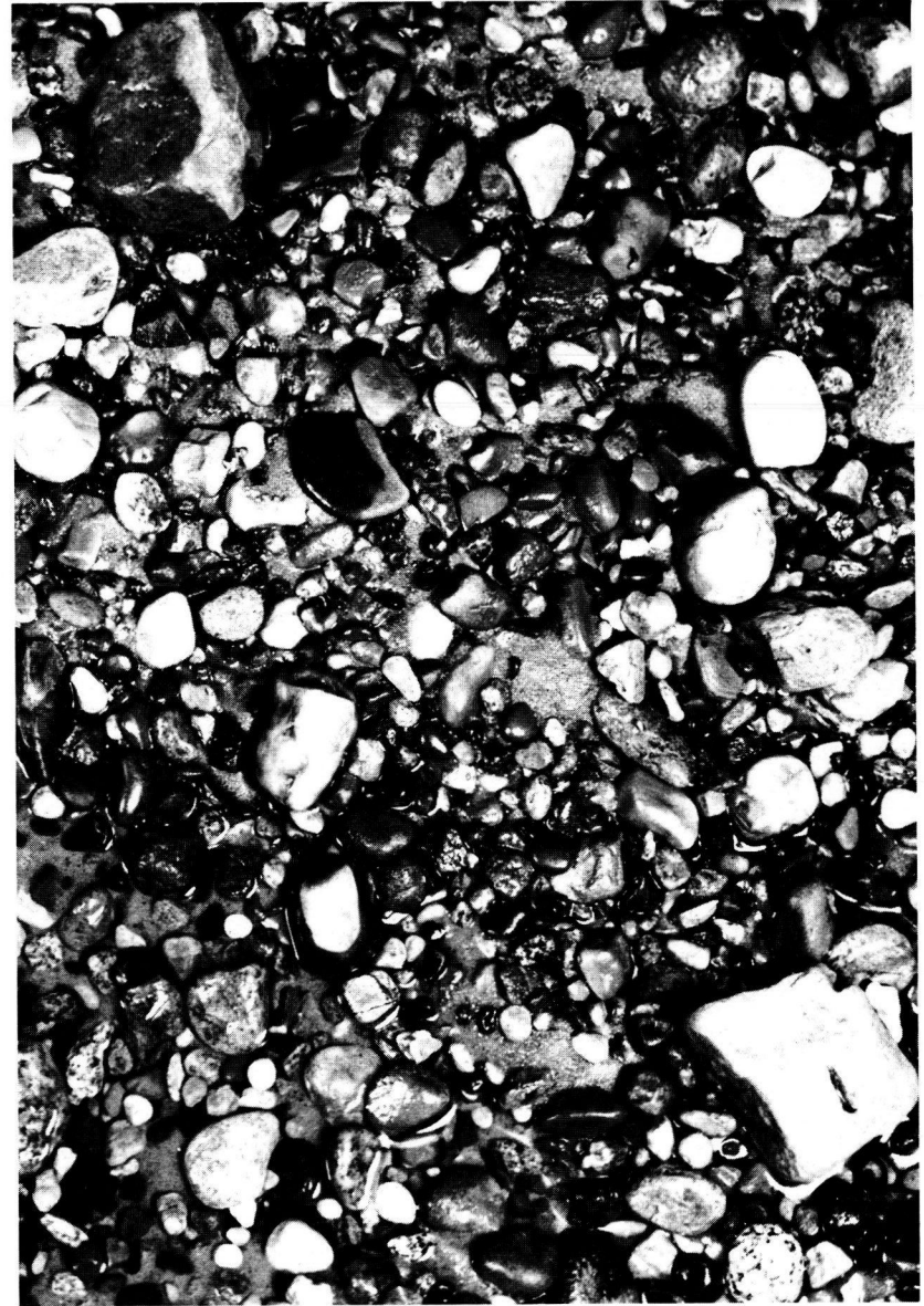
Figure 54. The area in Figure 53, but after an experiment of 51-min duration at the design flow. The larger particles appear to be undisturbed, but considerable movement of intermediate and smaller particles has taken place. The leaching of sand through the interstices by the flow is also apparent from the sand deposits on the riprap surface.
