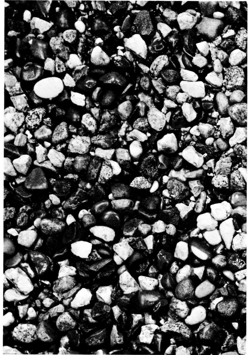
Figure 52. The bed in Figure 51, after the design discharge had been flowing over it for 9 hr. Because of the increased thickness, very little sand from the base has been removed and the bed is quite stable.
