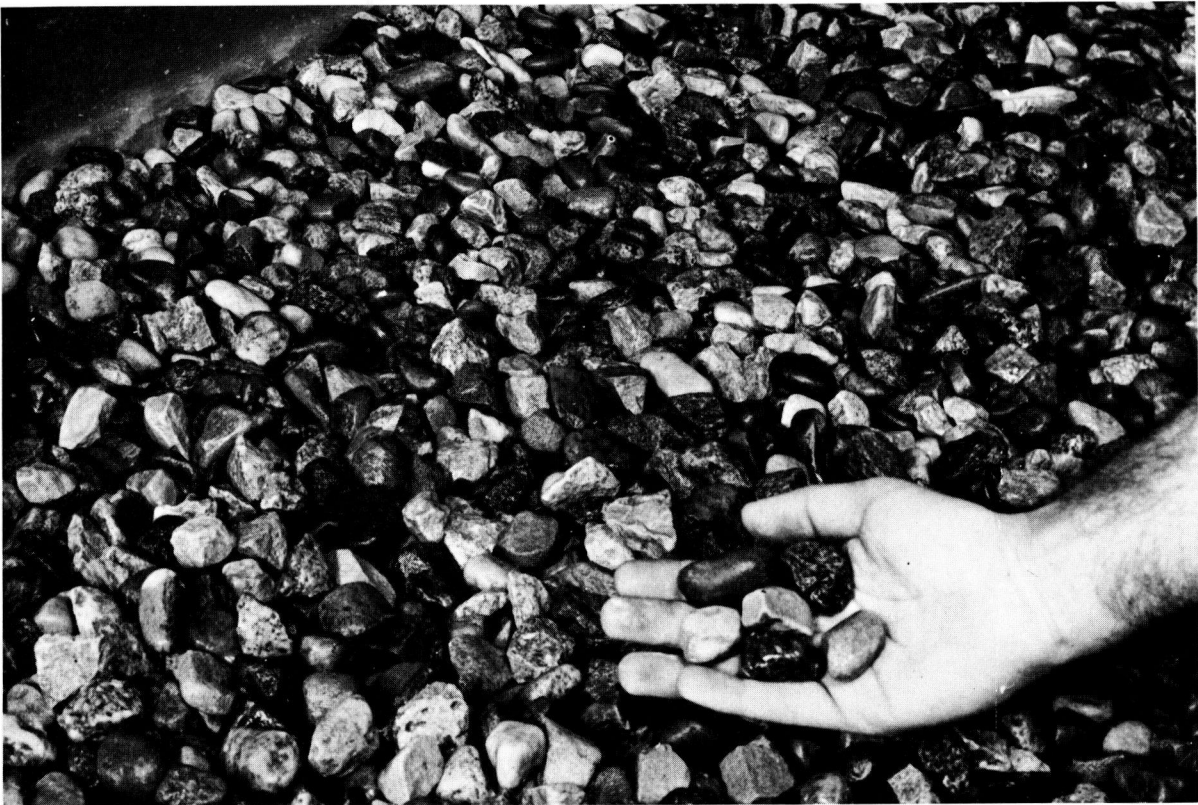
Figure 47. Uniform riprap material, showing size and shape of particles that have passed a 1-in. mesh sieve and have been retained on a \frac{3}{4} -in. mesh sieve.
