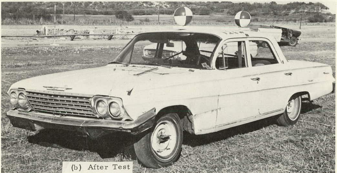
Figure A-4. Vehicle damage, Test 126.
