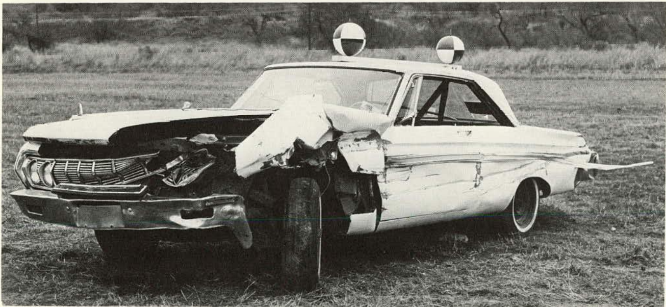
Figure A-11. Vehicle damage, Test 128.
