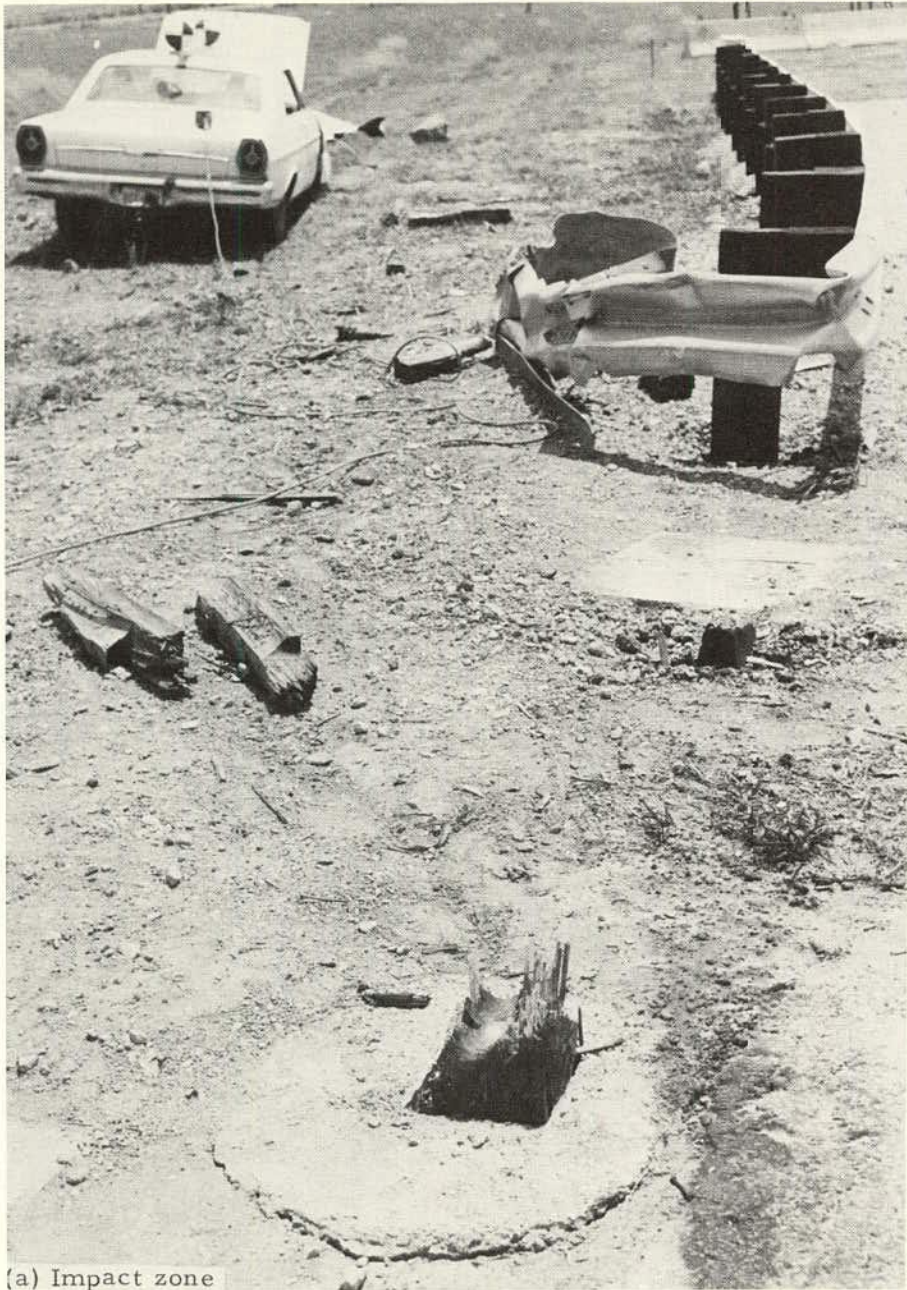
Figure A-23. Installation damage, Test 130.
