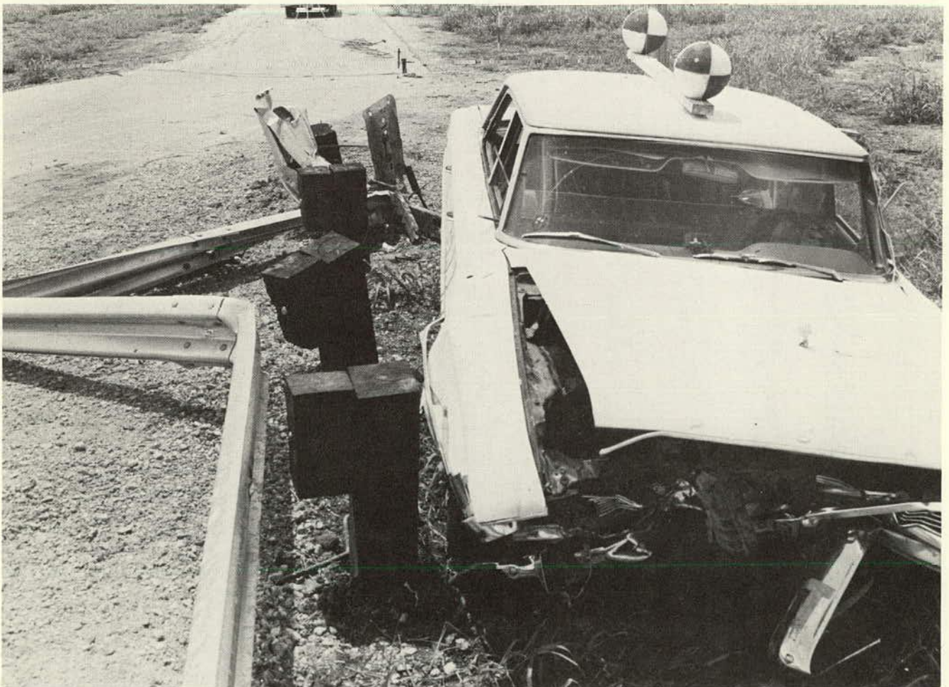
Figure A-31. Vehicle and installation damage, Test 132.
