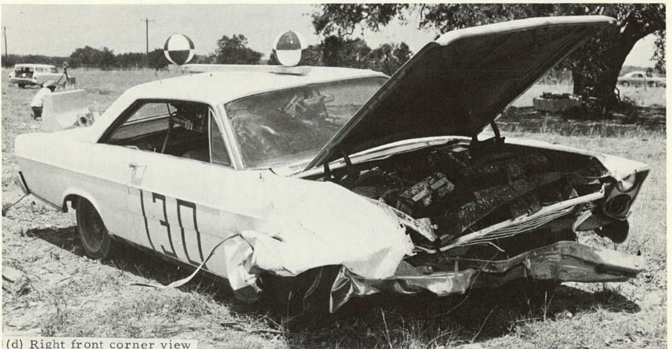
Figure A-25. Vehicle damage, Test 130.
