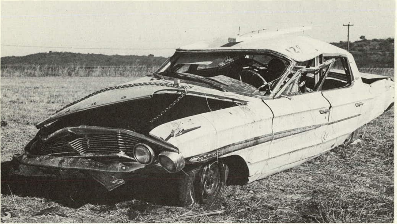
Figure A-16. Vehicle damage, Test 129.
