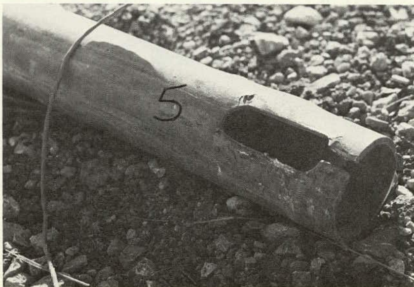
Figure A-15. Installation damage, Test 129.
