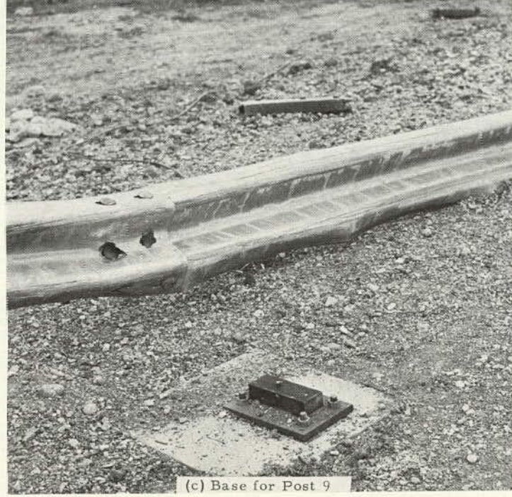
Figure A-10. Installation damage, Test 128.
