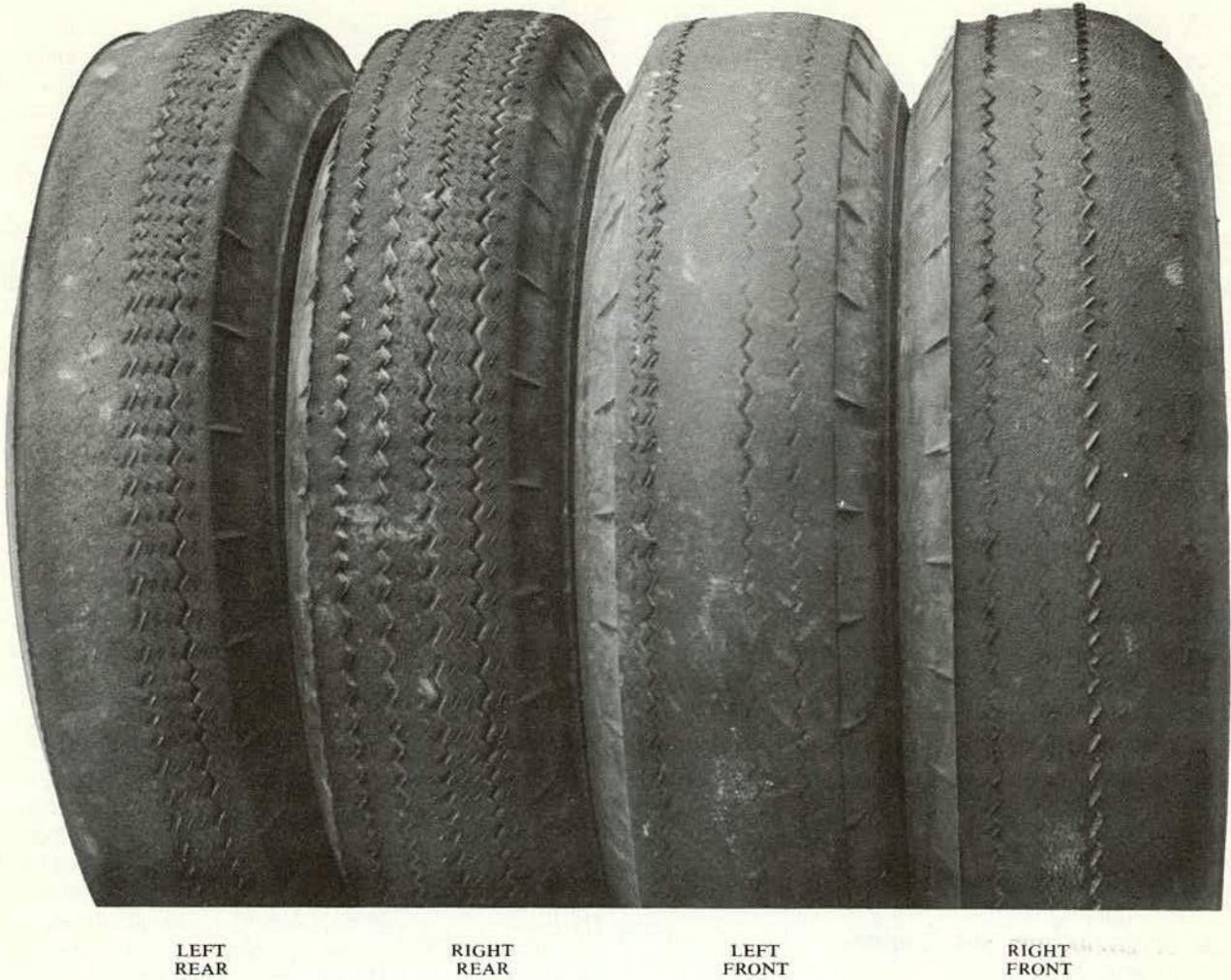
Figure 1. Pattern of tread wear of a set of tires for a passenger car driven 22 miles at 20 mph counterclockwise on a 65-ft radius circle, including 33 momentary stops. The right front and left rear tires are unusable, although each tire has only traveled 4,200 miles.
