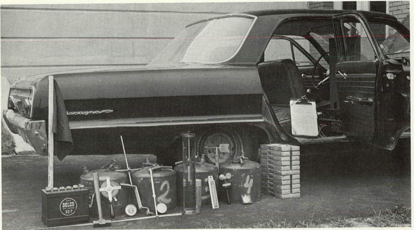
Figure 3. Special test equipment, including hand anemometer, hand wind vane, fuel hydrometer, and weights. The front of the fuelmeter is visible at the right of the driver's seat inside the vehicle.
