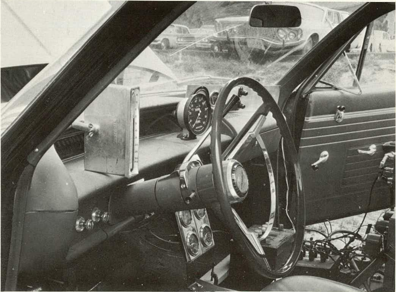
Figure 2. Interior of test vehicle, showing accelerometer, survey speedometer, manifold vacuum gauge, and engine temperature gauge. The back of the fuelmeter is visible to the right of the driver's seat. The tachometer and part of the manifold vacuum gauge are behind the steering column.
