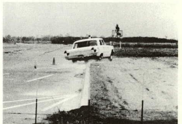
Figure D-19. Photographic comparison of Test N-7 HVOSM vehicle behavior with that of the full-scale-test vehicle on impact with curb Type E at 60 mph and a 12.5-deg angle in identical time sequences.
