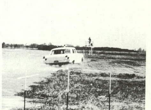
Figure D-20. Photographic comparison of Test N-18 HVOSM vehicle behavior with that of the full-scale-test vehicle on impact with curb Type C at 60 mph and a 12.5-deg angle in identical time sequences.
