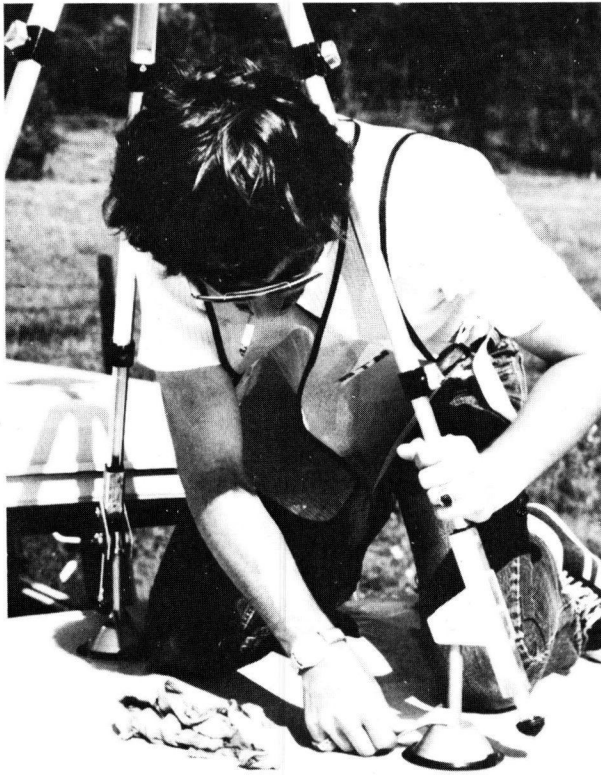
Figure 4. Positioning camera tripod with special suction pads on top of truck cab.
