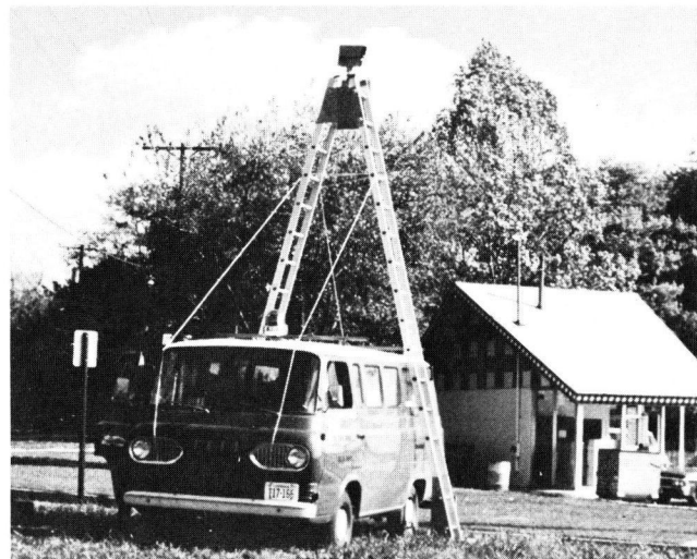
Figure 3. Time-lapse camera positioned on top of 15-ft A-frame ladders.
