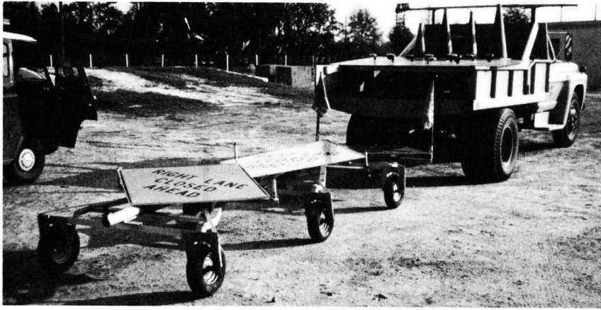
Figure 8. Sign train used to expedite placing traffic controls.
