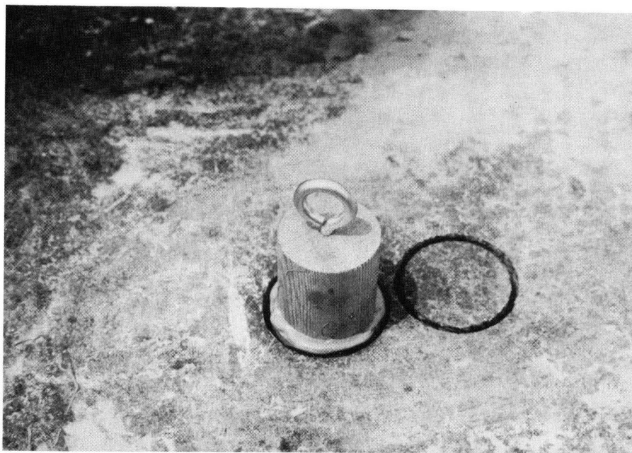
Figure C-2. Field bond test with cylindrical wooden block in place ready for testing (left). After testing, the core on right is removed by chiseling from the core hole on left.
