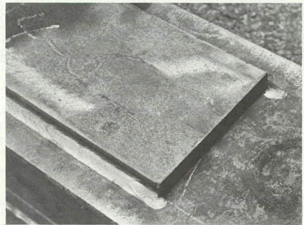
b) End of fillet weld.
