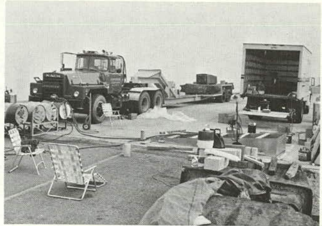
Figure H-11. Circulation of heater water from drums to impregnation chamber.
