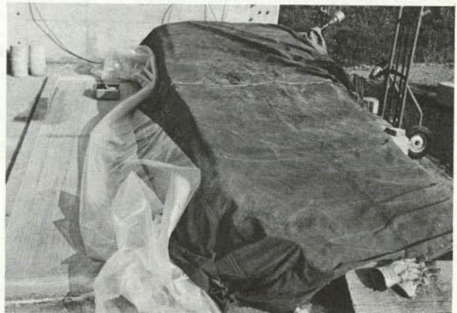
Figure H-13. View of chamber cover with insulation during hot-water polymerization.
