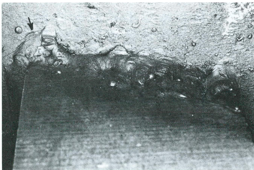
Figure 14. 0.25-in. (6-mm) crack at flange framed into web, groove welded.
