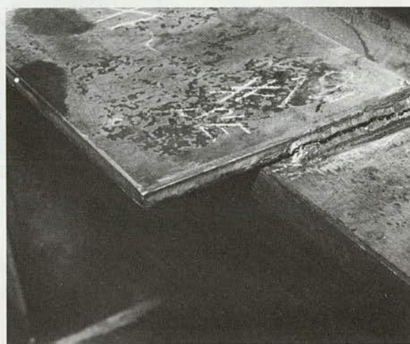
Figure 39. Weld crack through throat of fillet weld at root.
