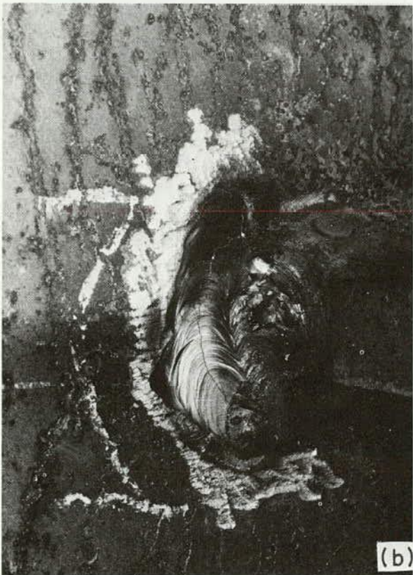
Figure 55. (a) Crack before GTA remelting; (b) crack after GTA remelting.
