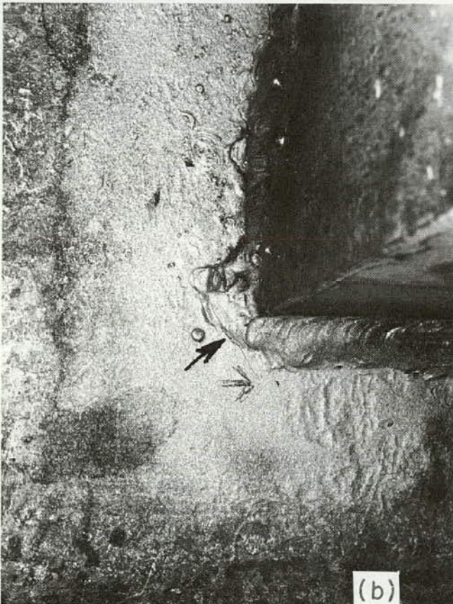
Figure 41. Cracks forming at ends of welded attachments: (a) crack at fillet weld toe; (b) cracks at groove weld toe.
