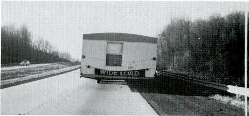
Figure 14. Typical encroachment of wide load onto paved shoulder along freeway.
