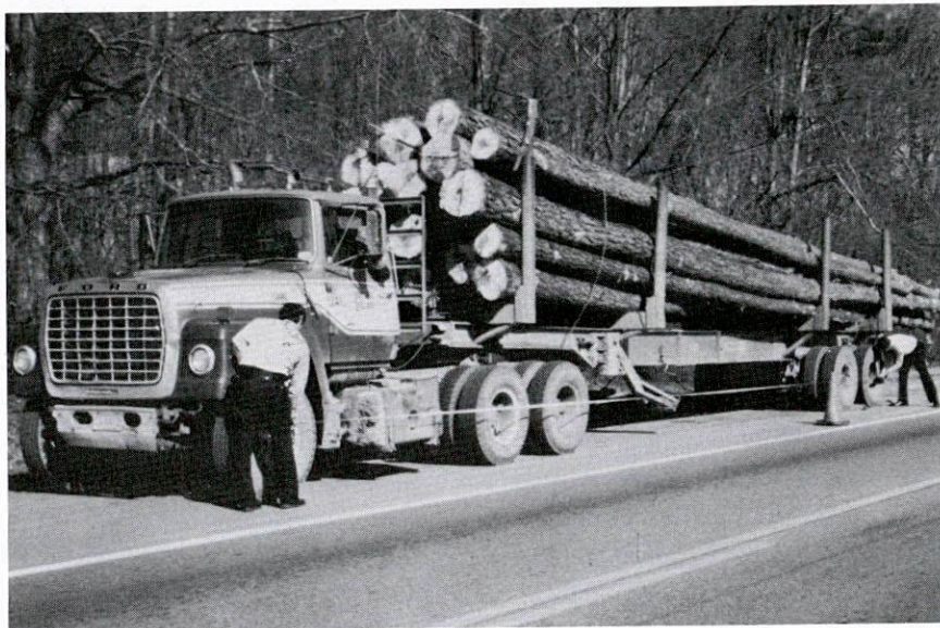
Figure 23. Use of specially constructed shoulder by enforcement agency to weigh (portable scales) and measure trucks.
