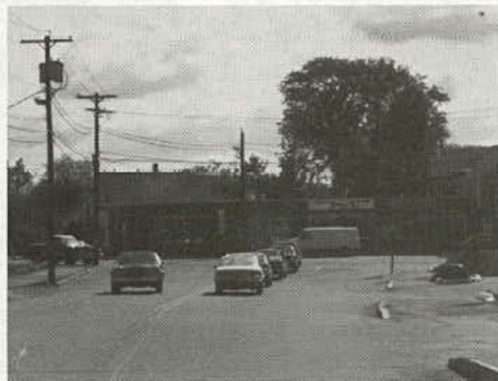
(e) The Clinton Street to South Street left turn operates at a poor level of service throughout the day. This heavy left turn operates under stop control, which creates substantial queues and long delays.
