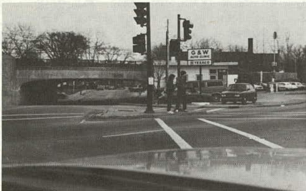
Large, raised traffic islands provide pedestrian refuge.
