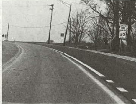
(a), (b) and (c) The bypass lane for westbound traffic begins about 300 feet in advance of the intersection. It is intended for optional use by through drivers who encounter queued left turning vehicles in the left lane. The bypass lane merges back into the through lane past the intersection.
