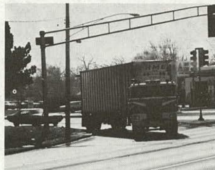
(d) and (e) Right turn roadway width and radius design enable easy turns by frequent semi-trailers.
