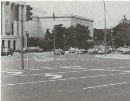
(a) and (b) Well-marked double left turn lanes and turn Constitution Avenue traffic into a 36-foot throat.
