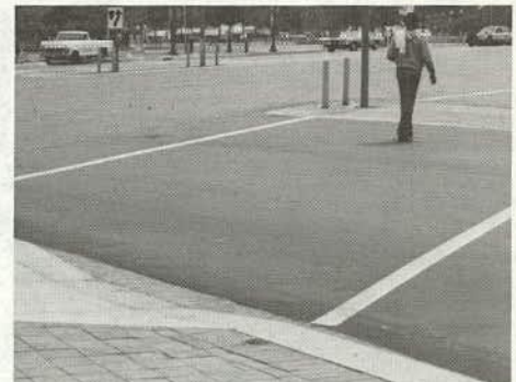
(e) and (f) Pedestrian movements across Pennsylvania Avenue are restricted to the 4th Street intersection, where pedestrian actuated signals are provided. Handicapped ramps are installed at all pedestrian crossings.
