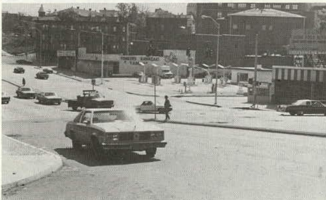
Raised medians of sufficient width are also used by pedestrians crossing wide arterials.
