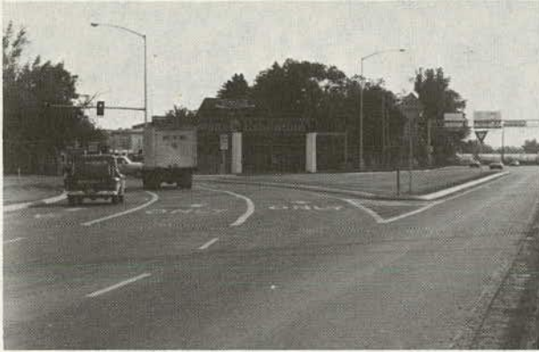
Traffic islands separate movements and define vehicle paths.
