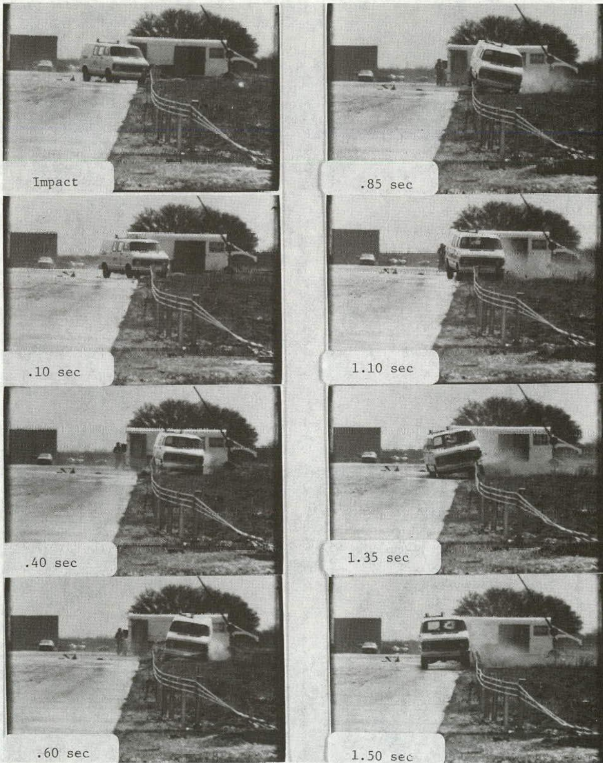
Figure 37. Sequential photographs as viewed from downstream of the barrier, test GR-17.
