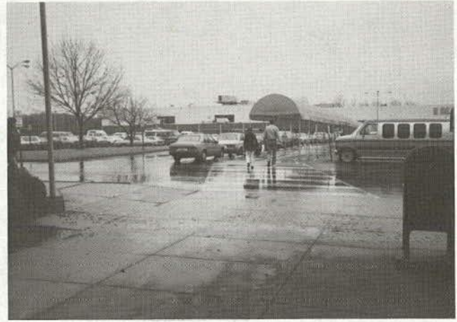
Figure 30. Covered walkway through a parking lot. (This canopy at the Plymouth Meeting Mall delineates the walkway location to both pedestrians and motorists.)
