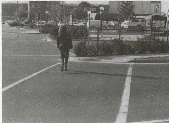
Pedestrian approach to Metro station is nicely landscaped, but awkward. Simple opening in fence could have alleviated this problem.
