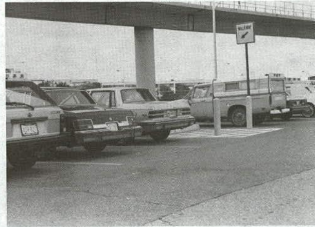
Visible signing placed over the tops of cars can help pedestrians to find their way through parking lots and other areas.
