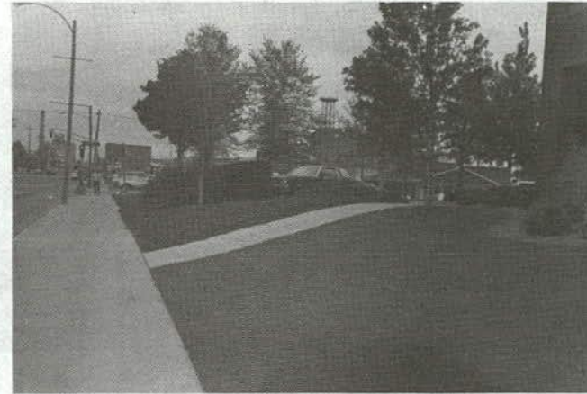
Pedestrian access should be provided where there are natural desire lines between buildings and the street.
