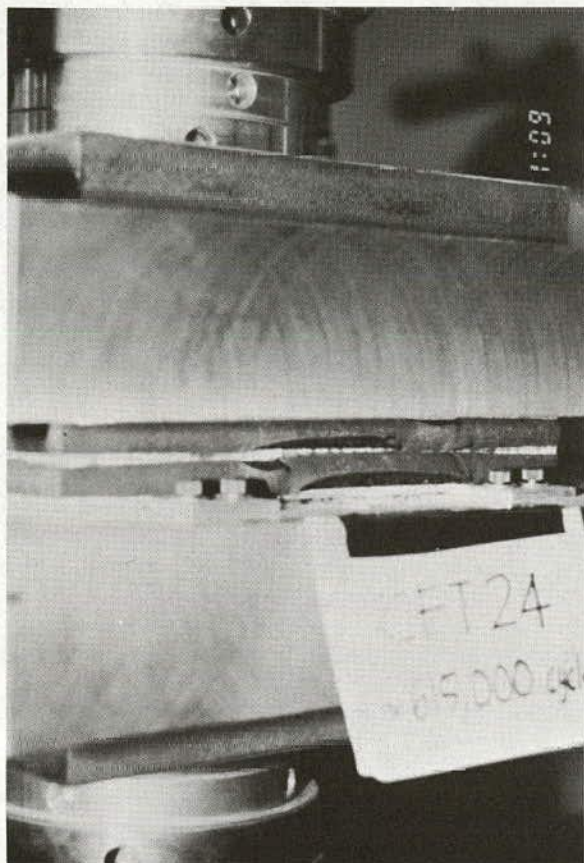
Figure F-15. Photograph of typical fatigue cracking from the compression fatigue tests.
