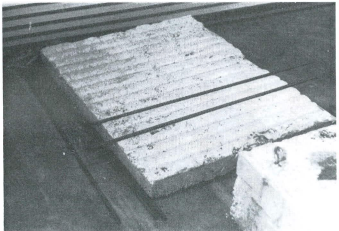
Figure F-6. Bottom of test slab with variable reinforcing steel spacing capability.
