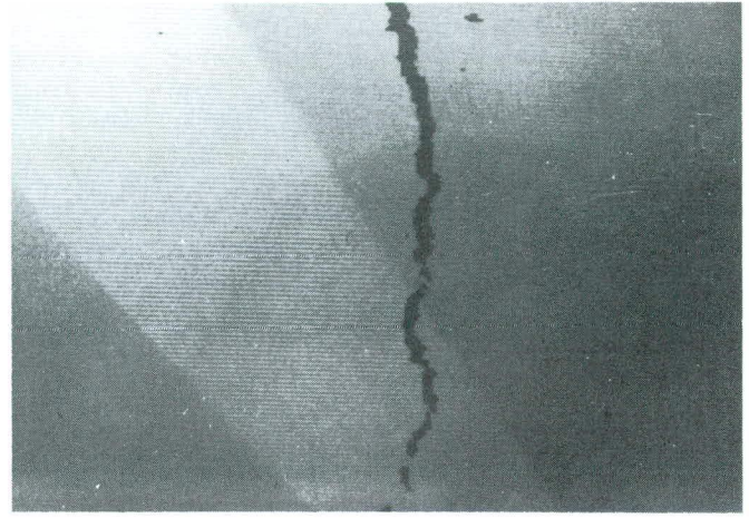
Figure D-3. Sample loading bay image with a threshold of 3 standard deviations below the mean.
