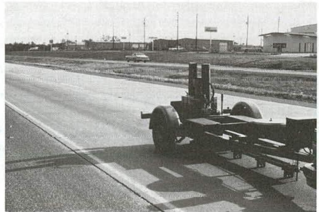
Figure 7. Dynatest falling weight deflectometer.
