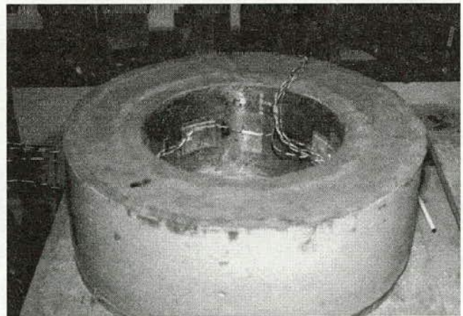
Figure 1. Cracking-tendency test apparatus (left—empty, right—full of concrete).
