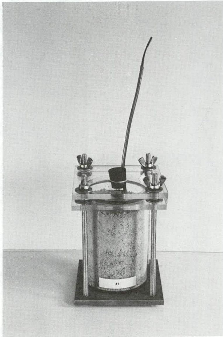
Figure E-1. Photographs of Soil Test Cells Containing Bentonite (Left) and Sand (Right) Used for Polarization Resistance Measurements.
