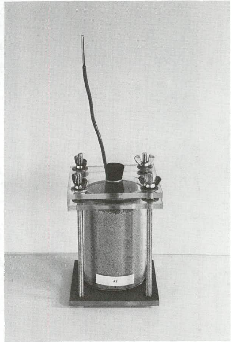
Figure E-1. Photographs of Soil Test Cells Containing Bentonite (Left) and Sand (Right) Used for Polarization Resistance Measurements.
