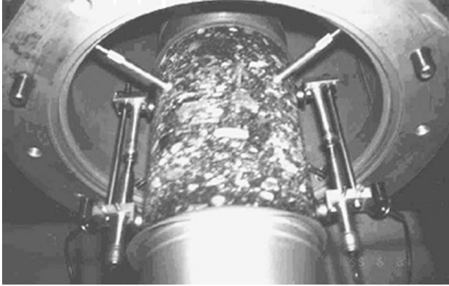
Figure 21. Vertical and radial LVDTs setup for an unconfined test.
