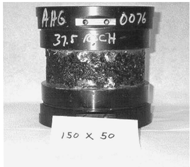
Figure 25. Test specimen prepared for testing with aluminum platens glued to top and bottom.
