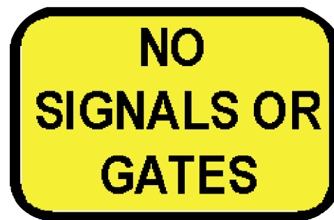
Figure 7. Supplemental plaque for passive crossings—Option 1.
