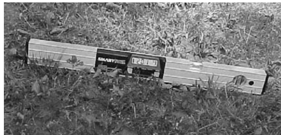
Figure 35. Measuring a Slope with a Digital Level
