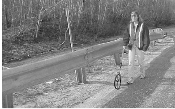
Figure 24. Measuring the Length of Barrier
