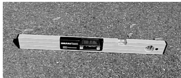
Figure 45. Estimating Grade with a Digital Level
