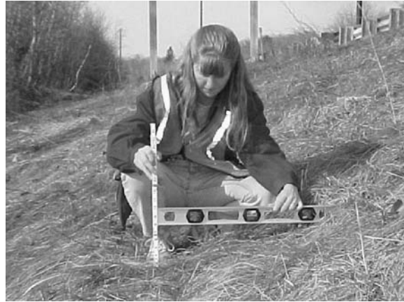
Figure 33. Measuring a Slope Behind a Barrier
