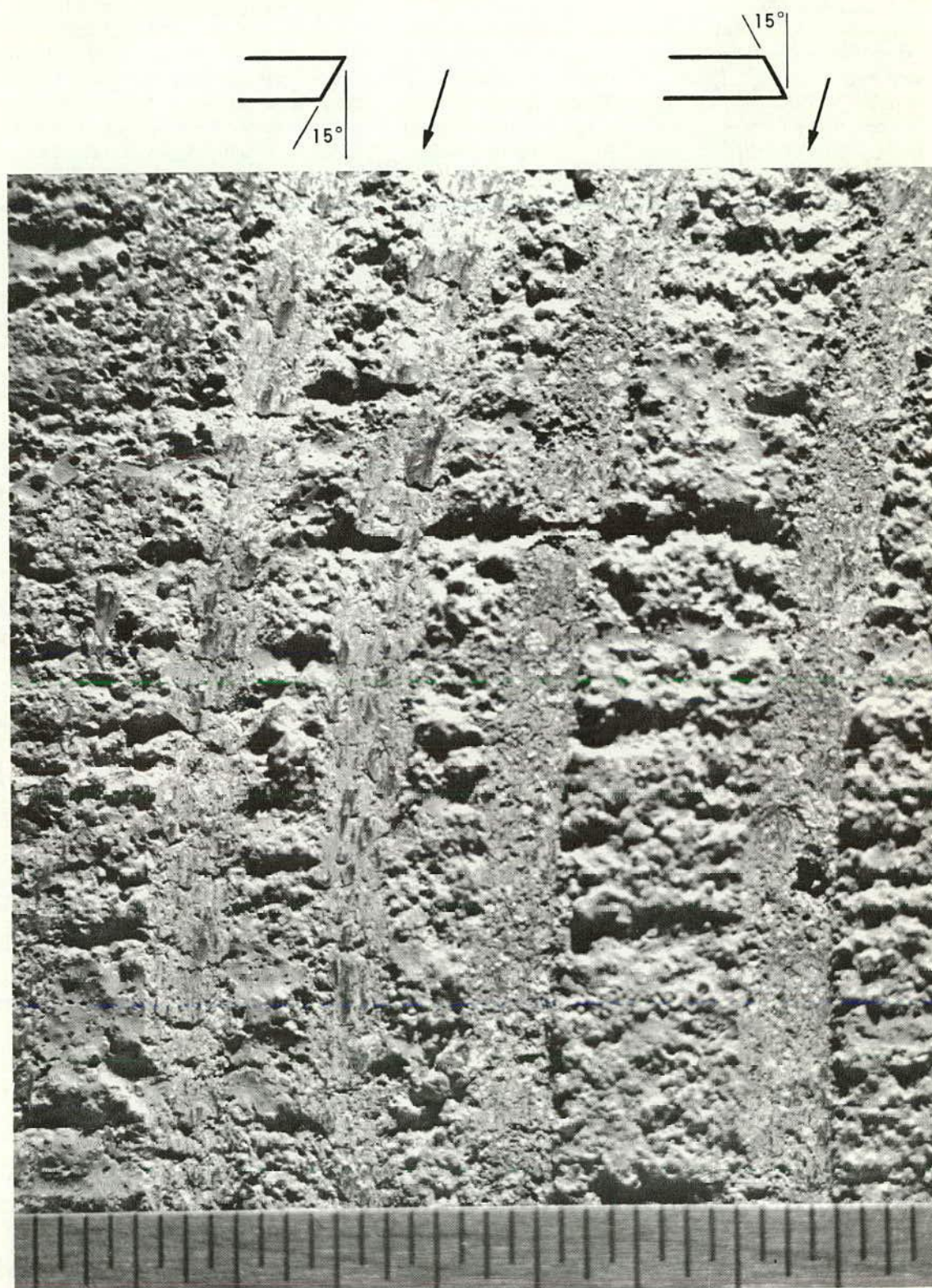
Figure B-9. Wear tracks by studs with various clearance angles.
