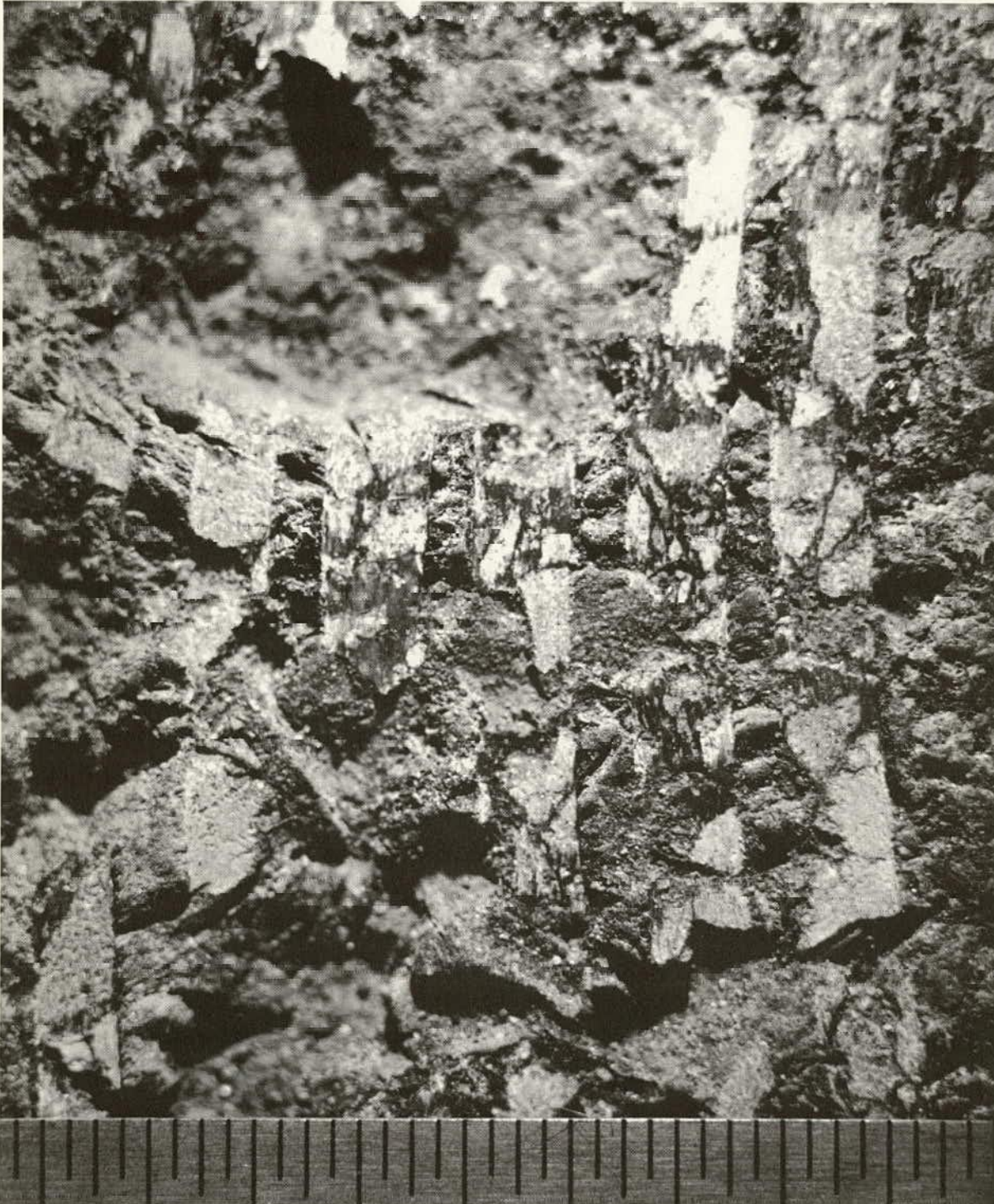
Figure B-6. Wear tracks in bituminous concrete.
