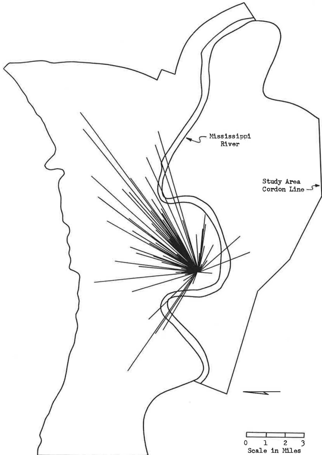
Figure C-3. Zonal interchange transit trip desire lines (unweighted by trip volumes) to a selected university in the New Orleans urban area, typical weekday, 1960.
