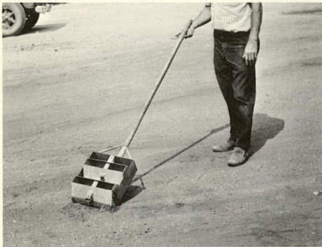
Figure 10. Asphalt Institute sampling device.
