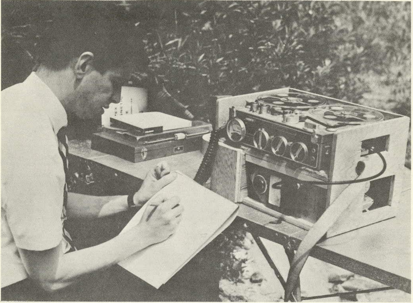
Figure B-2. Precision sound level meter (lower instrument) and instrumentation tape recorder (upper instrument) used in field measurements.
