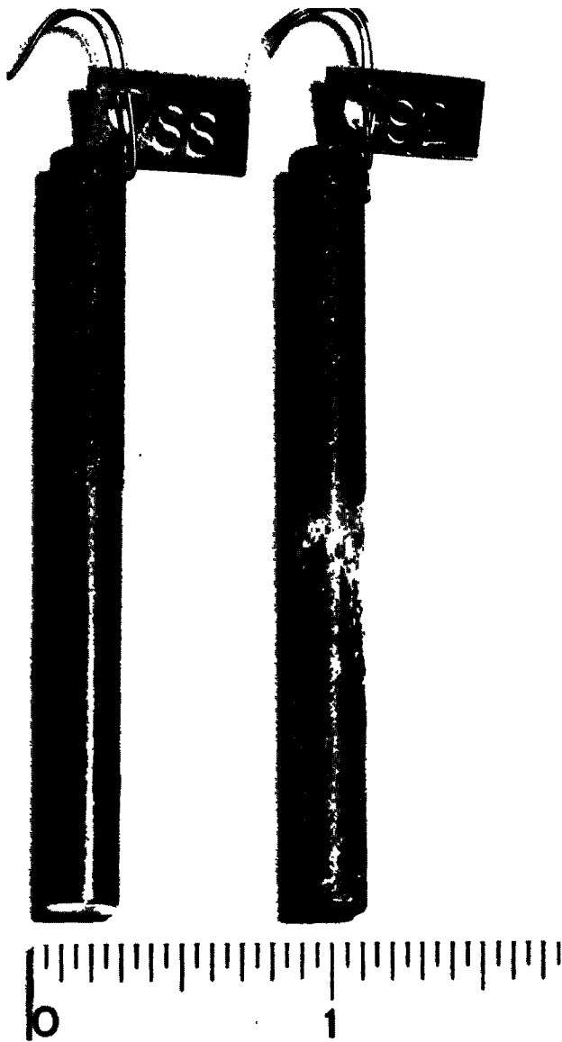
Figure E-14. Specimens after 800 hr in moisture condensation test. Lower half of Specimen 88 is coated with Shell water-soluble oil; lower half of Specimen 92, with sodium silicate-sodium nitrite coating, S-65.
