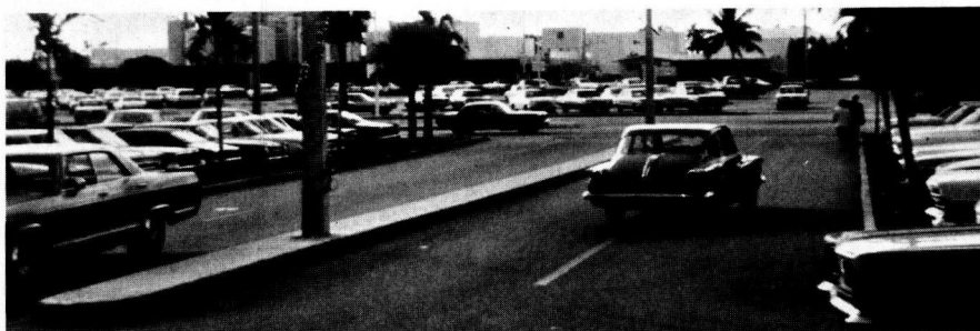
Figure 26. Extension of driveway into the parking lot of regional shopping center to promote orderly on-site circulation and free ingress/egress maneuvers.
