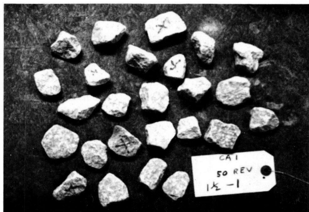
Figure B-5. Aggregate CA1, 1½-to-1-in. fraction after 50 drum revolutions.
