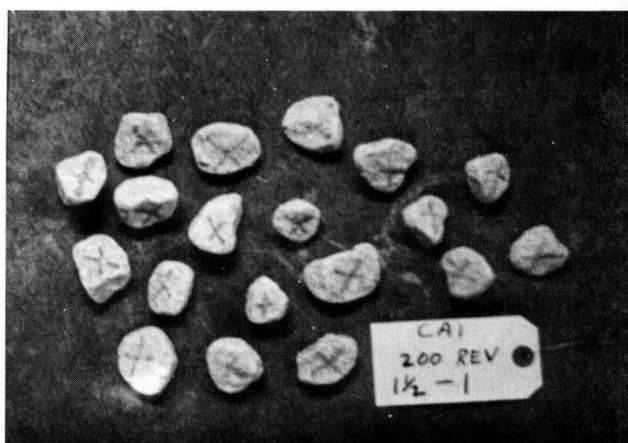
Figure B-7. Aggregate CA1, 1½-to-1-in. fraction after 200 drum revolutions.
