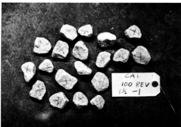
Figure B-6. Aggregate CA1, 1½-to-1-in. fraction after 100 drum revolutions.
