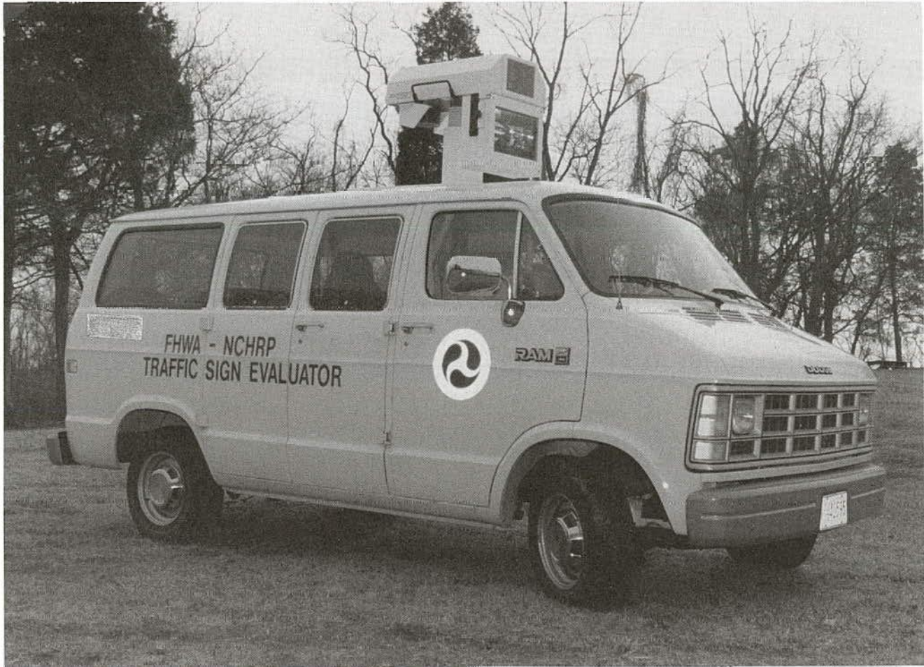
FIGURE 6 Prototype mobile retro-reflectivity measurement system.
