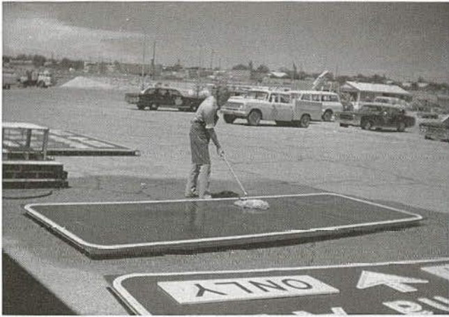
FIGURE 22 Sign blank rinsed and mopped dry.
