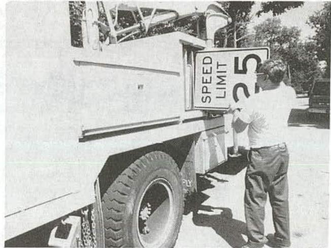
FIGURE 31 Sign storage on truck.
